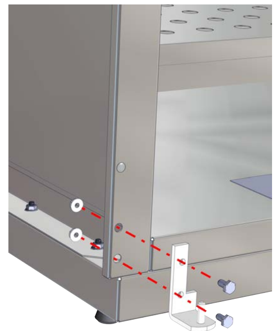
Fig. 65: Install Bottom Hinge in New Position
