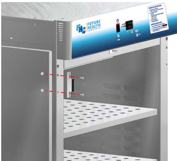
Fig. 55: Install Male Hinge Halves in New Position
