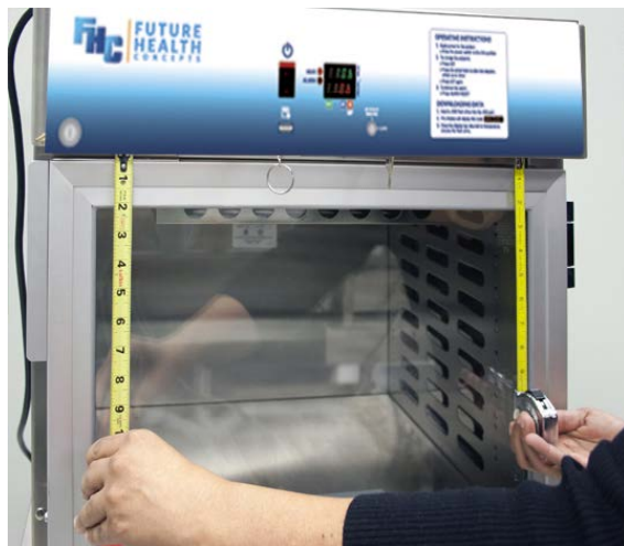
Fig. 68: Check Alignment - Square Door
