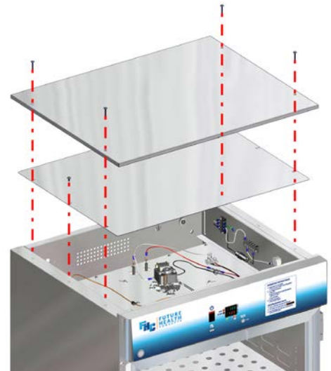
Fig. 29: Remove Top Panels
