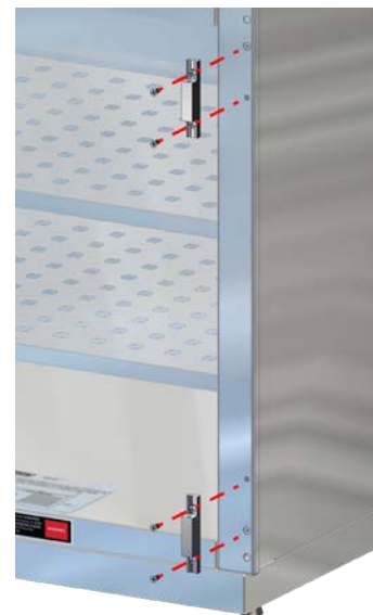
Fig. 46: Detach Glass Door Hinge - Male Half
