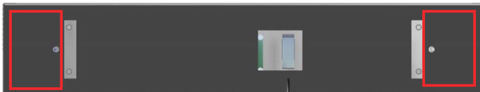
Fig. 34: Cut Out Rectangular Sections from Gasket
